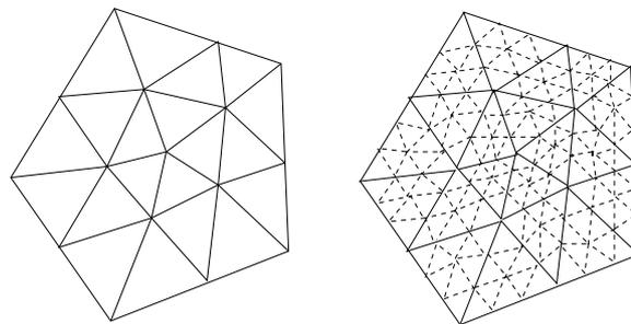
Figure 1: The coarse and refined grid partition
