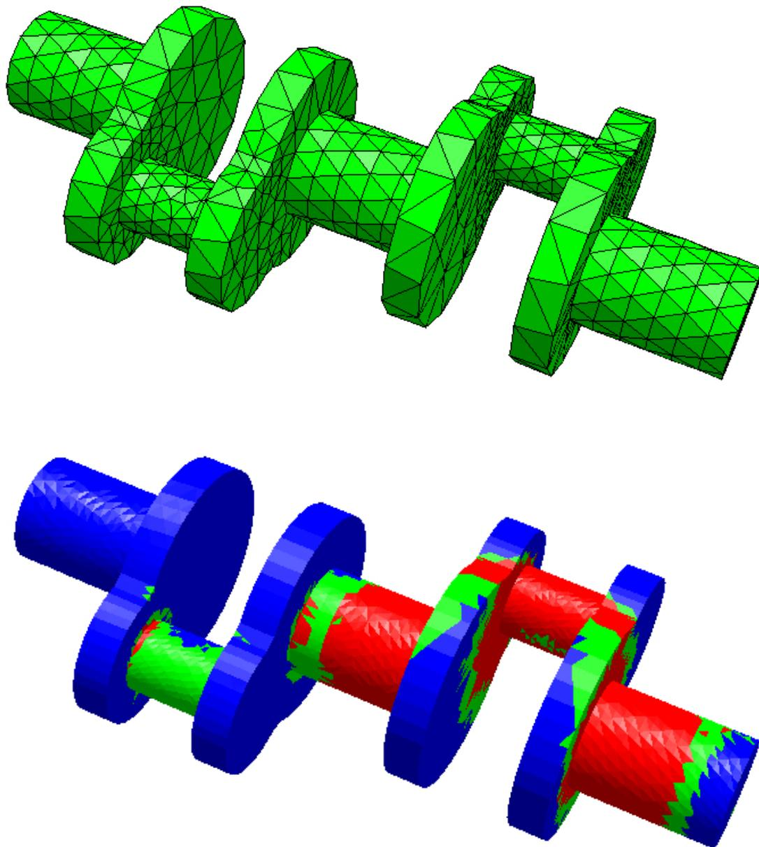
Figure 6: Geometry (top) and elastoplastic zones (bottom) in the numerical experiment with the two-yield crankshaft explained in Subsection 4.3. The blue color shows elastic zones, green and red color zones in the first and second plastic phase. Pictures were generated by NETGEN/NGSOLVE software [Sch].
