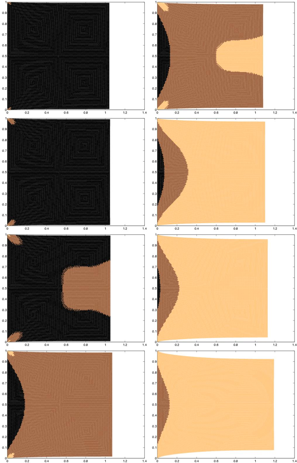
Figure 2: Evolution of elastoplastic zones at discrete times  $t = 4.5, 5, 5.5, 6, 6.5, 7, 8, 9$  in the numerical experiment with the two-yield 2D beam explained in Subsection 4.2. The black color shows elastic zones, brown and lighter gray color zones in the first and second plastic phase. A corresponding movie can be found in [ani].
