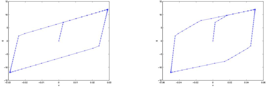
Figure 4: Displayed loading-deformation relation in terms of the uniform surface loading  $g_x(t)$  versus the  $x$ -displacement of the point  $(0, 1)$  for problems of the single-yield 1D beam (left) and two-yield 1D beam (right).
