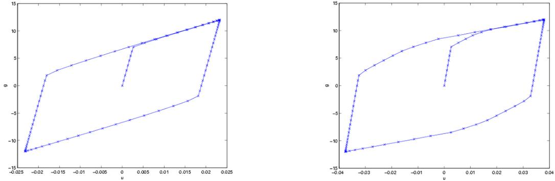
Figure 5: Displayed loading-deformation relation in terms of the uniform surface loading  $g_x(t)$  versus the  $x$ -displacement of the point  $(0, 1)$  for problems of the single-yield beam with 2D effects (left) and two-yield beam with 2D effects (right).
